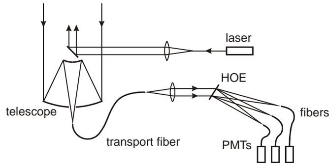
**Fig. 1:** The basic lidar system. A laser beam is expanded, collimated and directed into the atmosphere. The return light is collected by a transport fiber at the focus of the telescope. The light exiting the fiber is collimated and passed through the HOE to isolate RRS and Rayleigh light into individual fibers for photon counting in photomultiplier tubes (PMTs).
