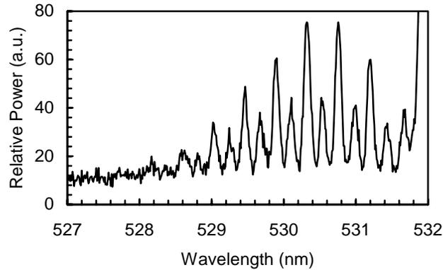
**Fig. 4:** RRS spectrum. This shows a plot of the nitrogen, anti-Stokes RRS spectrum made by scanning a 50 $\mu$ m multimode fiber along the focal plane of the HOE. The excitation laser (532nm) was directed into a nitrogen cell at 10 atmospheres.
