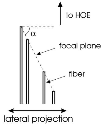
**Fig. 3:** Fiber positioning. The fibers are placed along an angled focal plane to collect the focused light at each RRS line. Shown here are the fibers for the J=20, 16 and 6 RRS lines, along with another for the Rayleigh line (left to right).
