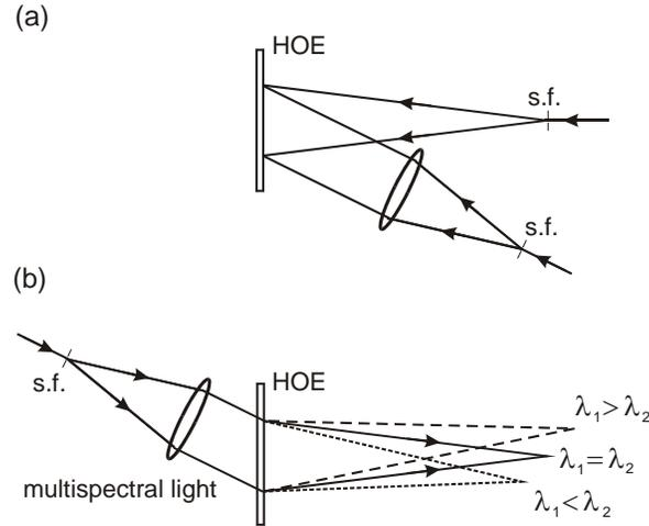
**Fig. 2: a.** Recording. The hologram is recorded between a divergent beam (from spatial filter, s.f.) perpendicular to the plate and a plane wave reference beam incident from an angle. **b.** Reconstruction. The phase conjugate reference beam at wavelength  $\lambda_2$  will focus at a different spatial location relative to the recording wavelength ( $\lambda_1$ ).
