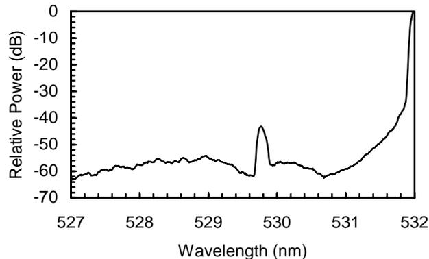
**Fig. 5:** Scattered light. The plot of the relative power scattered into a 50 $\mu$ m multimode fiber along the focal plane of the HOE illuminated by the recording laser ( $\lambda = 532$ nm). The secondary peak near 530nm results from a front back reflection within the hologram.
