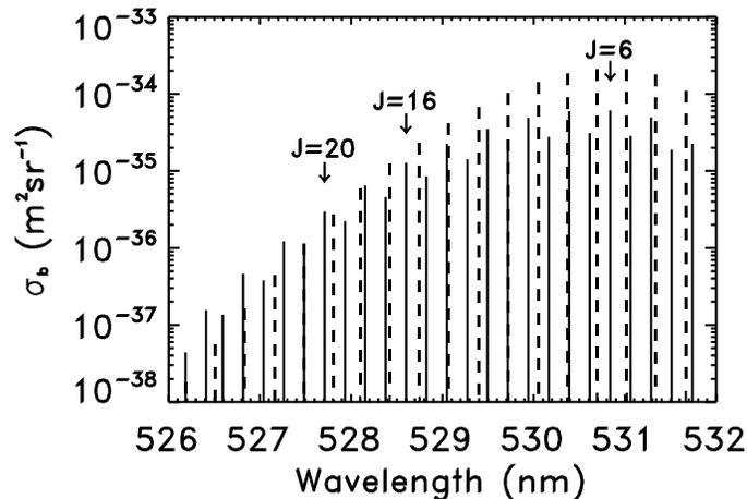
**Fig. 6:** The predicted rotational Raman spectrum. A plot of the 250K, RRS anti-Stokes backscattered cross-section ( $\sigma_b$ ) for both O<sub>2</sub> (dashed) and N<sub>2</sub> (solid), at an excitation wavelength of 532.075nm. The N<sub>2</sub> lines at J = 6, 16 and 20 are indicated.
